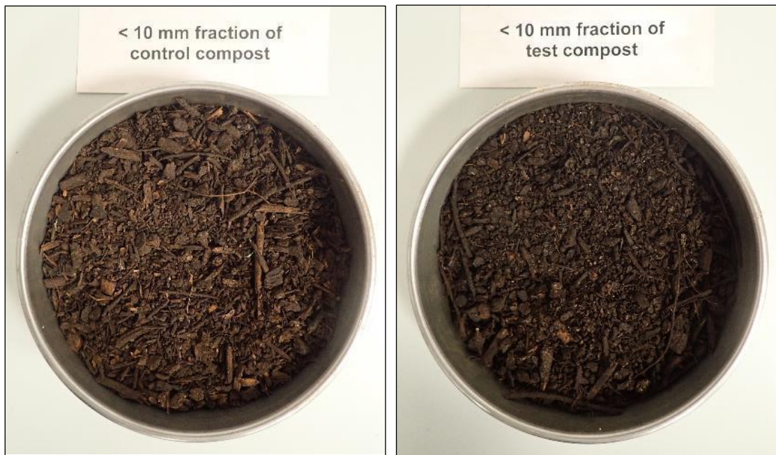
Figure 15. Visual comparison between the < 10 mm fraction of control compost and test compost obtained after 12 weeks of composting
