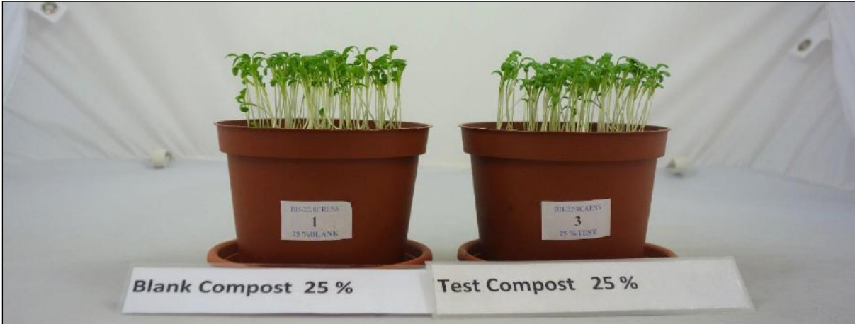
Figure 5. Detailed cress plant growth after an incubation period of 7 days (from left to right): 25% series of blank compost and test compost
