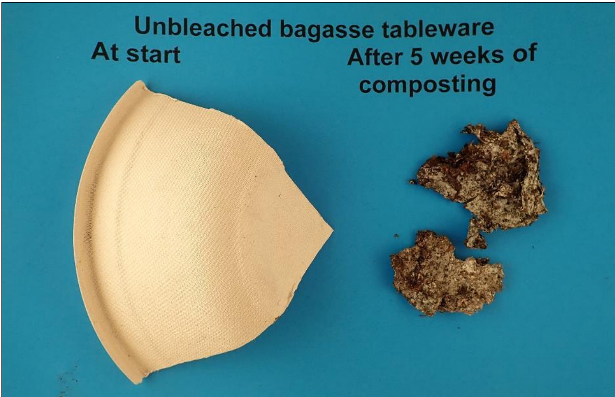
Figure 13. Visual comparison between test item Unbleached bagasse tableware (thickness: 0.92 mm (bottom), 1.04 mm (side); grammage: 629 g/m 2 (bottom), 476 g/m 2 (side)), cut into 4 pieces, at start and after 5 weeks of composting
