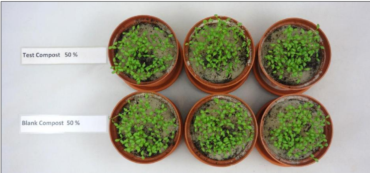
Figure 6. Overview of the cress plant growth after an incubation period of 7 days (from bottom to top): 50% series of blank compost and test compost
