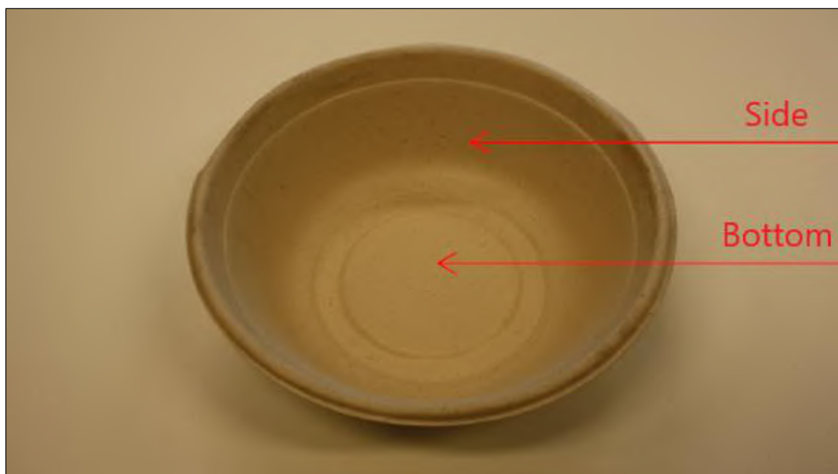
Figure 3. Measurement points on Unbleached bagasse tableware (Side and Bottom)
