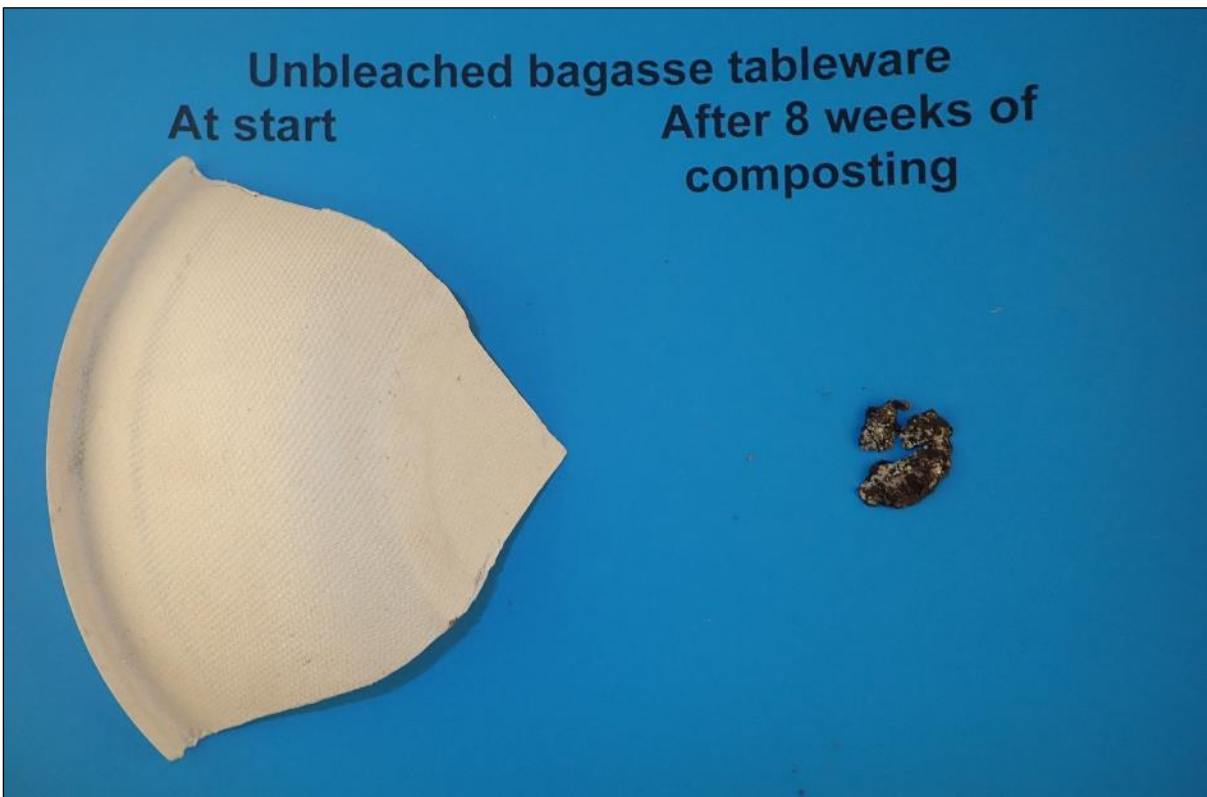
Figure 14. Visual comparison between test item Unbleached bagasse tableware (thickness: 0.92 mm (bottom), 1.04 mm (side); grammage: 629 g/m 2 (bottom), 476 g/m 2 (side)), cut into 4 pieces, at start and after 8 weeks of composting
