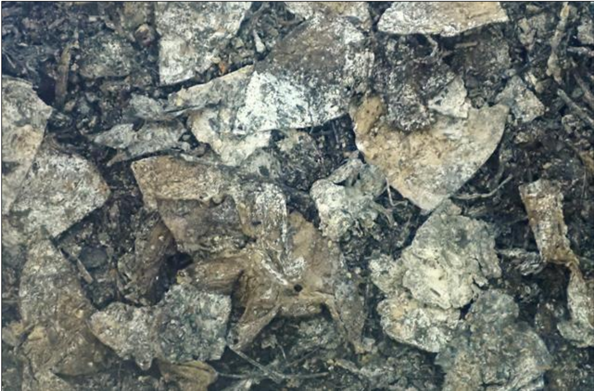
Figure 11. Visual comparison between test item Unbleached bagasse tableware (thickness: 0.92 mm (bottom), 1.04 mm (side); grammage: 629 g/m 2 (bottom), 476 g/m 2 (side)), cut into 4 pieces, at start and after 3 weeks of composting
