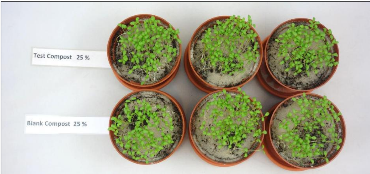
Figure 4. Overview of the cress plant growth after an incubation period of 7 days (from bottom to top): 25% series of blank compost and test compost
