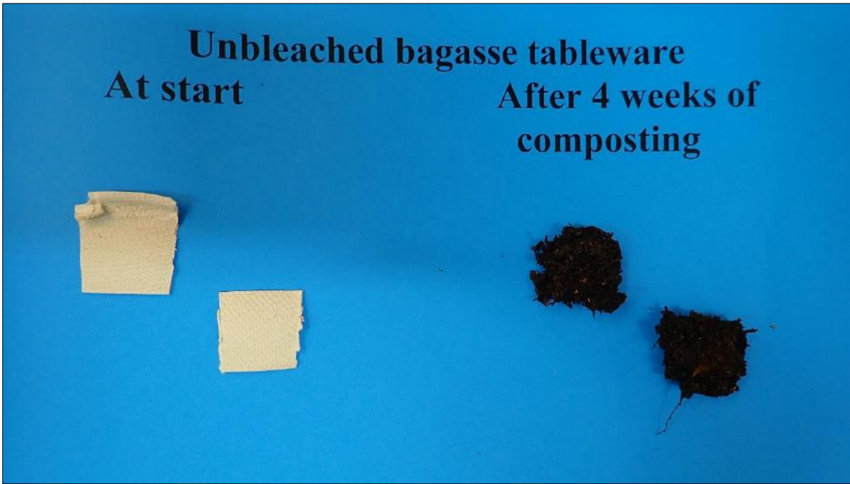
Figure 3. Visual comparison between Unbleached bagasse tableware, cut into 2.5 cm × 2.5 cm pieces, at start and after 4 weeks of composting
