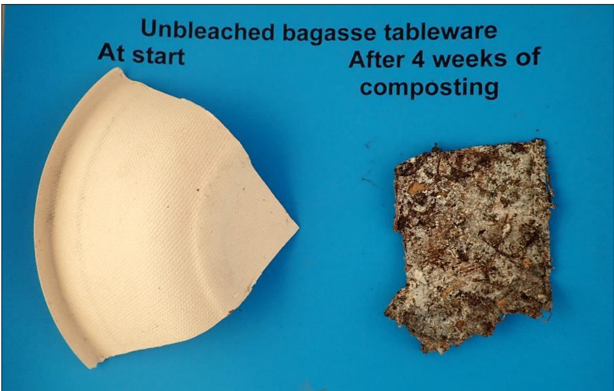
Figure 12. Visual comparison between test item Unbleached bagasse tableware (thickness: 0.92 mm (bottom), 1.04 mm (side); grammage: 629 g/m 2 (bottom), 476 g/m 2 (side)), cut into 4 pieces, at start and after 4 weeks of composting
