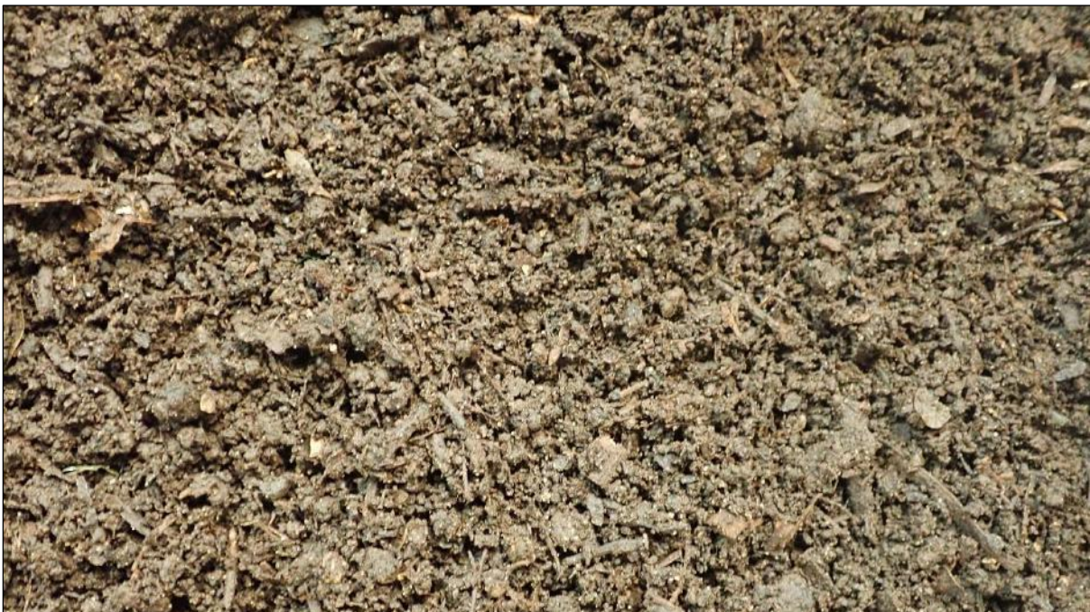
Figure 4. Visual presentation of a composting reactor with Unbleached bagasse tableware after 8 weeks of incubation at ambient temperature
