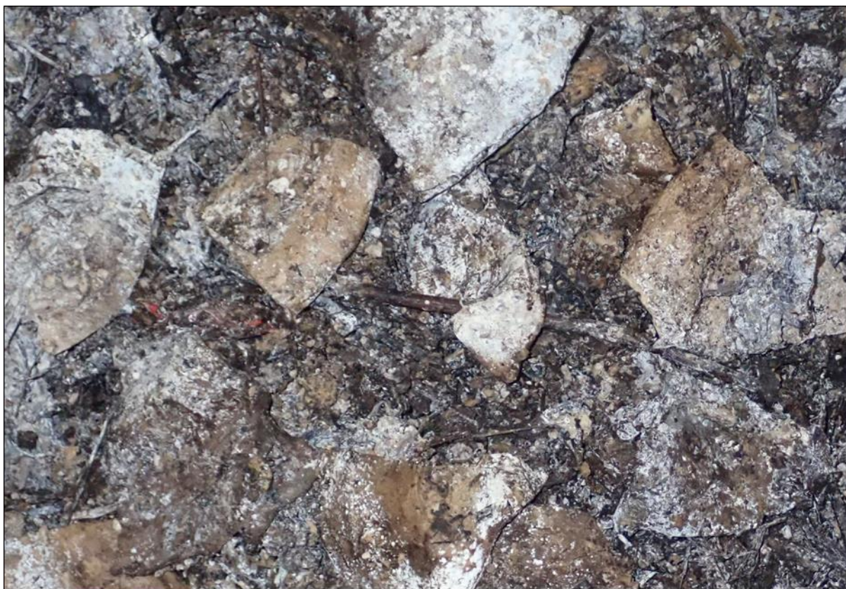
Figure 10. Visual presentation of the contents of a test bin with 1% Unbleached bagasse tableware (thickness: 0.92 mm (bottom), 1.04 mm (side); grammage: 629 g/m 2 (bottom), 476 g/m 2 (side)), cut into 4 pieces, and 9% Unbleached bagasse tableware (milled < 4 mm) after 2 weeks of composting
